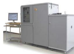
Field cycling relaxometer designed to measure the field dependence of T_1 from 0.01MHz to 1 tesla (42.6 MHz) [9]
