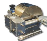
The 2.2 Tesla, iron-yoked split-pair high temperature superconducting magnet, cooled by a single stage Gifford-McMahon cryorefrigerator.
